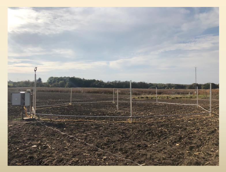
Each ring is constituted by a control unit and a series of 8 laser drilled pipes to release CO2. The release system is made by one storage tank holding the supply of liquid CO2 at -180° C, radiators bringing the gas to ambient temperature and a vaporizer that ensures non-interrupted supply of CO2 to the rings through underground pipes.
