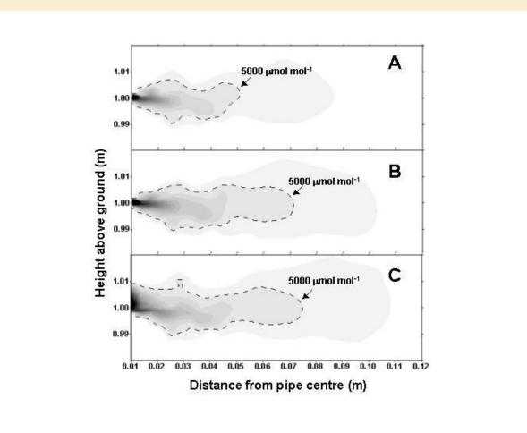
Furthermore, the microscopic holes (0.2mm diametr) laser-drilled into the outer circumference of these pipes, allow CO2 to be ejected out at sonic speed against the incoming air mass to maximise mixing of CO2 with ambient air.
