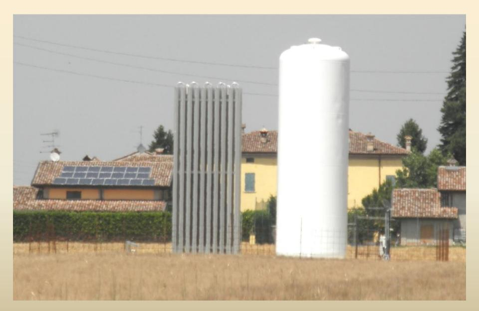
The release of CO2 is controlled through a system of valves connected to the 8 laser drilled pipes forming the sides of the ring itself. The pipes are installed on adjustable supports, which allow to raise the ring during the vegetation growth.
